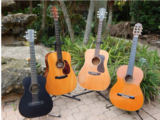
Fig. 1. From left to right: Martin LX (high pressure laminate – B&S, T; Stratabond® laminated birch – N); Martin D-18GE (Honduran mahogany B&S, N, Adirondack spruce – T); Guild 37BI (laminated hard maple arched – B, hard maple – N, S, Sitka spruce T, side); Takamine 132S (Indian rosewood B&S, western red cedar – T, Honduran mahogany neck), where B=back, N=neck, S=sides, and T=top).
